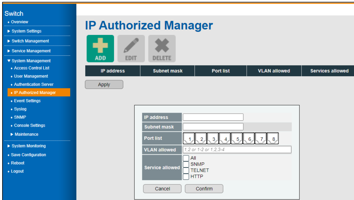
Figure 42 System Management > IP Authorized Manager Menu
